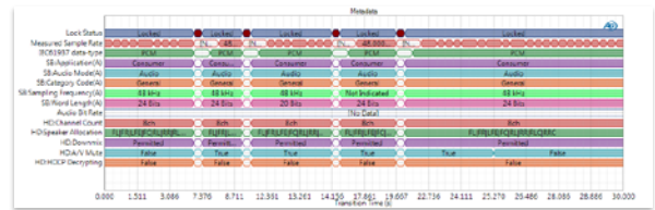
HDMI Metadata Monitor showing hotplug errors in-stream
