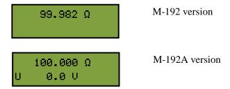
In the upper row generated resistance in  $[\Omega]$  is displayed. In the lower row mesaured voltage connected to the output terminals (M-192A only) is displayed.
