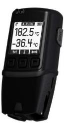
The EL-GFX-DTC standalone USB data logger measures and stores up to 252,928 temperature readings from two J, K, or T-type thermocouple inputs at a resolution of 0.1°C. Using the Windows control software (available as a free-download from www.easylogusb.com), users can quickly set up the data logger and view downloaded data by connecting the device to the PC's USB port using the supplied cable.
