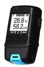
The EL-GFX-2 standalone USB data logger measures and stores up to 252,928 temperature and humidity readings over a -30 to +80°C (-22 to 176°F) and 0 to 100%RH range at a resolution of 0.1°C and 0.1%RH. Using the Windows control software (available as a free download from www.easylogusb.com), users can quickly set up the data logger and view downloaded data by connecting the device to the PC's USB port using the supplied cable.
