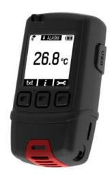
The EL-GFX-1 standalone USB data logger measures and stores up to 252,928 temperature readings over a -30 to +80°C (22 to +176°F) range and at a resolution of 0.1°C. Using the Windows control software (available as a free-download from www.easylogusb.com), users can quickly set up the data logger and view downloaded data by connecting the device to the PC's USB port using the supplied cable.
