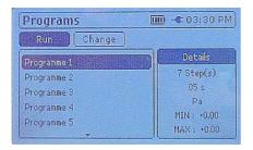
The Program function allows to defince the number and the duration of the different stages to reach. It is possible to save up to 20 different programs with 20 setpoints values (stages) by programm.
