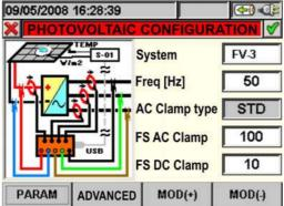
A synoptic connection scheme on the display helps the user while connecting the instrument to the installation (Single or Three phase) under
