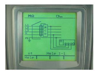
Help on line (available on each function) to support the user while connecting the instrument to the installation under measurement
