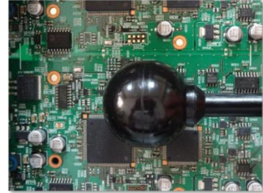
General sphere electric probe, diameter: 3cm
