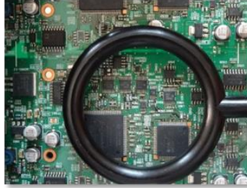
General loop magnetic probe , diameter: 6.8cm
