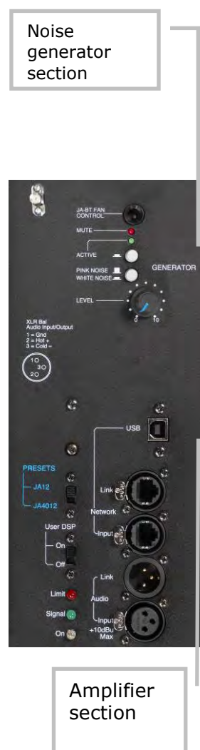
Fig. 2 – Generator section (above) and amplifier section (below) panel
