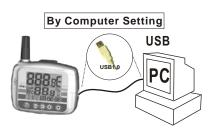
The meter canlink with computer to set the logging parameters which are introduced in Page5~Page11.
