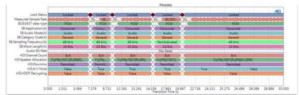
HDMI Metadata Monitor showing hotplug errors in-stream
